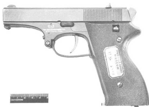
FIG. 9—Hi-Standard Model T-3 pistol, USA, Cal 9 mm Para, one retarding annular groove.
